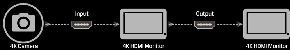
Equipped with HDMI 2.0 input/output interfaces, it can support up to 4096×2160 60p & 3840×2160 60p signal.
